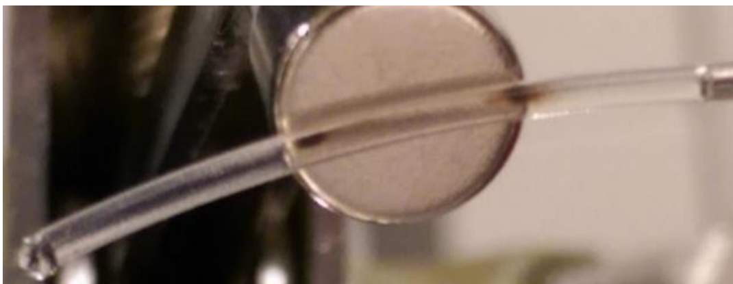
Figure 3.6 Fe 3 O 4 /SiO 2 /PMAA SPIONs captured in 0.6 mm inner diameter tube at 20 mm/sec flow rate.
